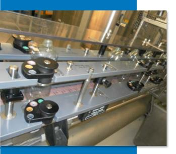
Similar to our other parts these conveyor guiderails are generally manufactured in 316 stainless steel and UHMWpe and are custom designed to suit specific containers
